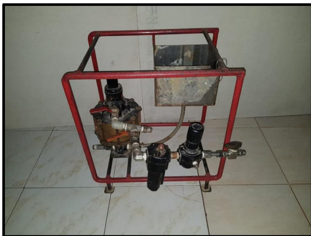
SC PUMP AIR DRIVENT MAX PRESSURE 10.000 PSI
