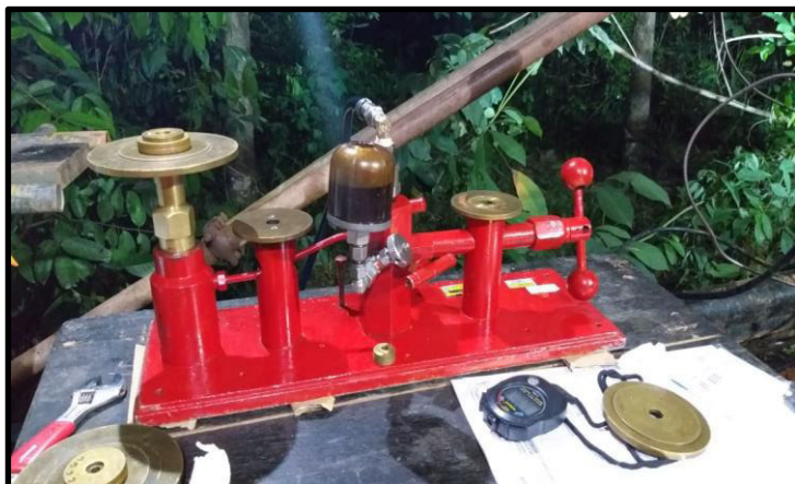
DEAD WEIGHT TESTER, MAX PRESSURE 10.000 PSI
