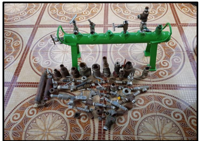
MANIFOLD TESTING MAX PRESSURE 10.000 PSI
