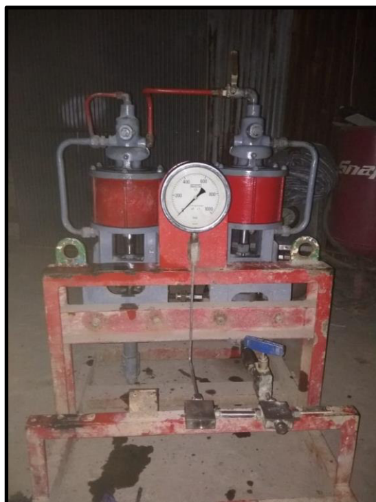
PNEUMATIC PUMP, MAX 10.000 PSI (HASKEL AIR DRIVENT)
