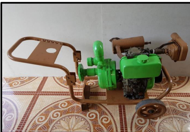
FILLING WATER PUMP 500 LITER / MINUTES MAX PRESSURE 200 PSI
